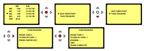
To delete one or more takes, select in the directory the lowest take number that needs to be deleted, press the 'CENTER' button (13) and select the 'TAKE ERASURE' menu. Once the selection confirmed by pressing the "CENTER" button (13), the erasing starts.
